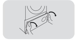
2. Turn the handle anti-clockwise and pull out the front cover.
