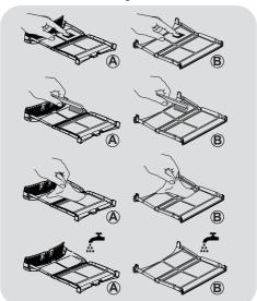
**4.** Close both filters by repositioning them inside the door, making sure they are positioned correctly in place.
