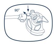
iii. Twist the plant protector to an angle of 90°.
