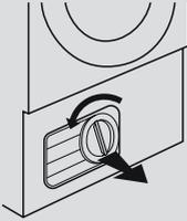
3. Gently clean the heat exchanger using a soft brush or a vacuum cleaner, to remove any dust or fluff, paying attention to not damage the fins.
