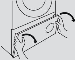
2. Turn the handle anti-clockwise and pull out the front cover.
