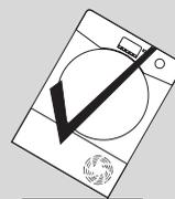
**If the product is in different side, wait at least 4 hours before switching on so that the oil can flow back into the compressor. Failure to do this could result in damage to the compressor.**
