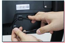
Plug in power cord to DC input and place excess cord in wire clip.
