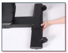
Place the front foot with wheels facing forward under the front bracket.
