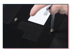
Remove the four preinstalled screws and set to the side.
