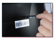
Unscrew the three small preinstalled screws from the cover on the back of the tablet and set aside. Flip the tablet back over.
