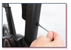
Insert handlebar post screw into hole on post. Use small hex key to tighten. Ensure holes in handlebar post and handlebar post frame align properly before inserting handlebar post bolt.
