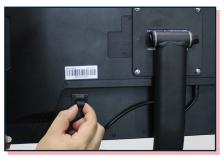
Place wire clip, as shown above, and press and hold wire clip down for ten seconds for proper adhesion.
