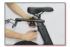
Pull and hold the seat height adjustment lever and raise the seat to desired position. Ensure lever engages one of the adjustment holes. Turn seat height adjustment lever clockwise until secure.
