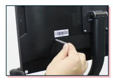
Replace the three screws to secure the cover back on the tablet.
