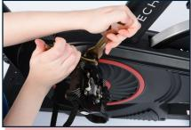
Hold pedal with double sided wrench and use single sided wrench to tighten nut counterclockwise.
