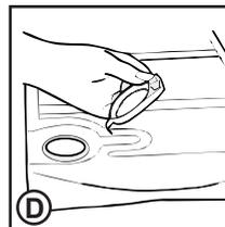
5. Refit the kickplate by engaging the hinges at the top and 'snapping' the lower clips into place.
