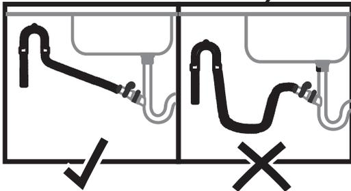
Ensure drain hose is routed straight to joiner. Remove excess drain hose material if necessary. Do not shorten the inlet hose.
