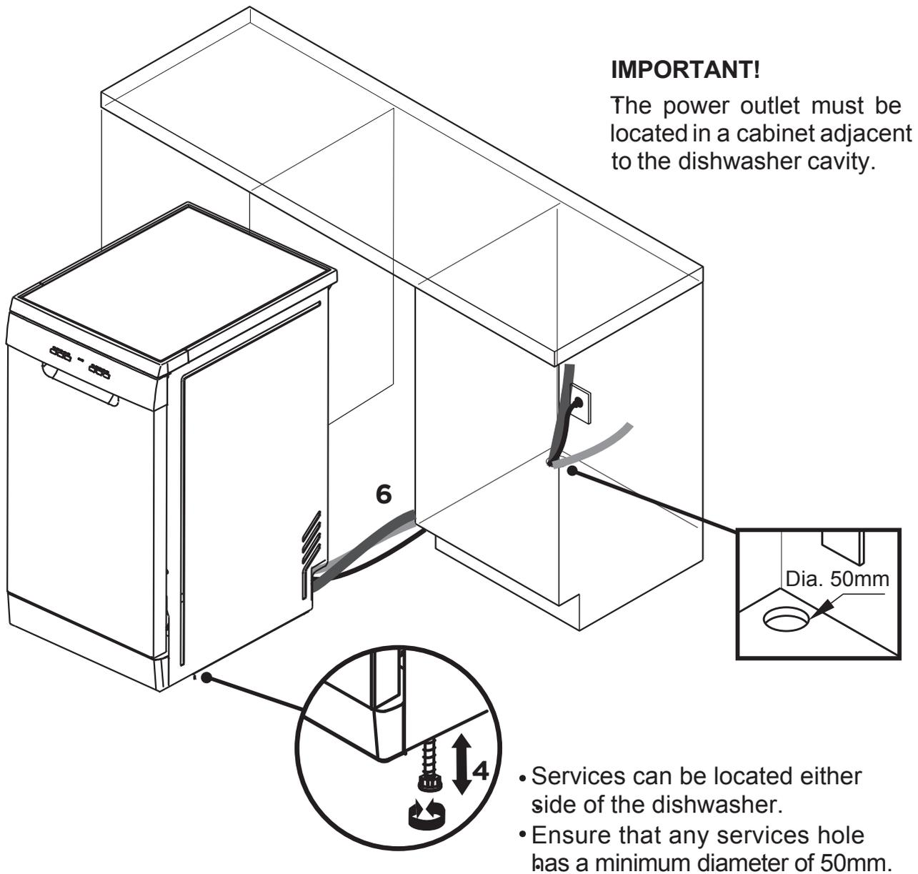
**3 Plumbing and drainage options. Determine which is more suitable**
