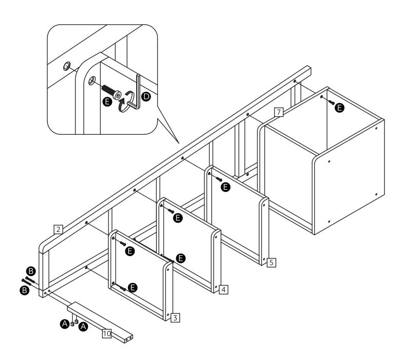
M10X12mm Nuts x2 M6X50mm Bolt x2 M6X25mm Bolt x10
