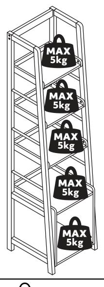
• WARNING: To prevent possible overbalancing this unit must be secured to a wall using the overbalance protector kit supplied.
