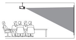
2 To adjust projection to the correct position, when the projector is turned on, press () on the projector to access the settings menu, then navigate to select *Proj. Direc. – Rev. front proj.*, then press **OK**.
