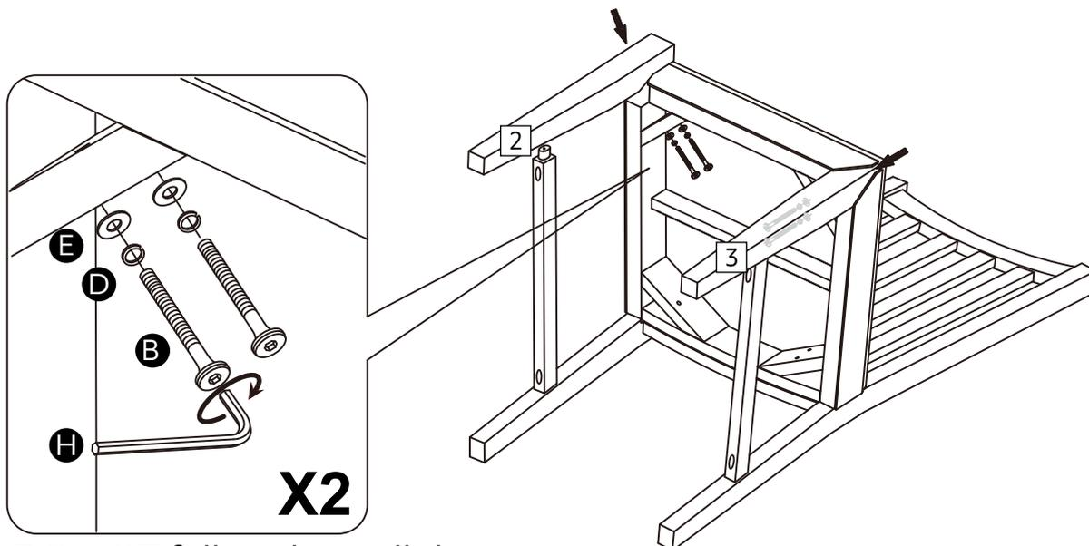
DO NOT fully tighten all the screws until assembly is completely finished
