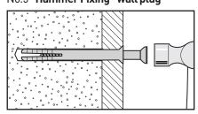
For use with walls stuck with plasterboard. The hammer fixing allows it to be fixed to the wall rather than the plasterboard. Always check the fixing is secure to the retaining wall.
