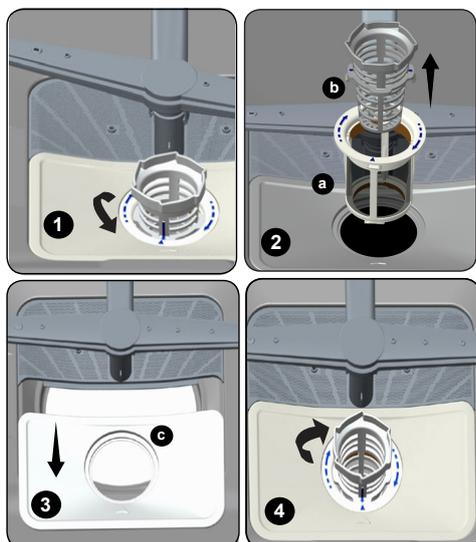
To remove and clean the filter combination, turn it counter clockwise and remove it by lifting it upwards (1). Pull the coarse filter out of the micro filter (2). Then pull and remove the metal filter (3). Rinse the filter with lots of water until it is free of residue. Reassemble the filters. Replace the filter insert, and rotate it clockwise (4).
