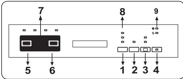
You can press the On/Off button (4) to switch on the product. On/Off lights will be on so long as the machine is on. Press the program button (5) to set the suitable program.
