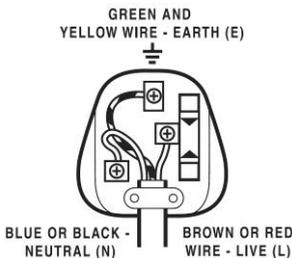
The BLUE wire must be connected to the terminal marked with the letter N
