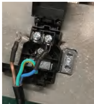
Fasten the wires beneath the screw heads
