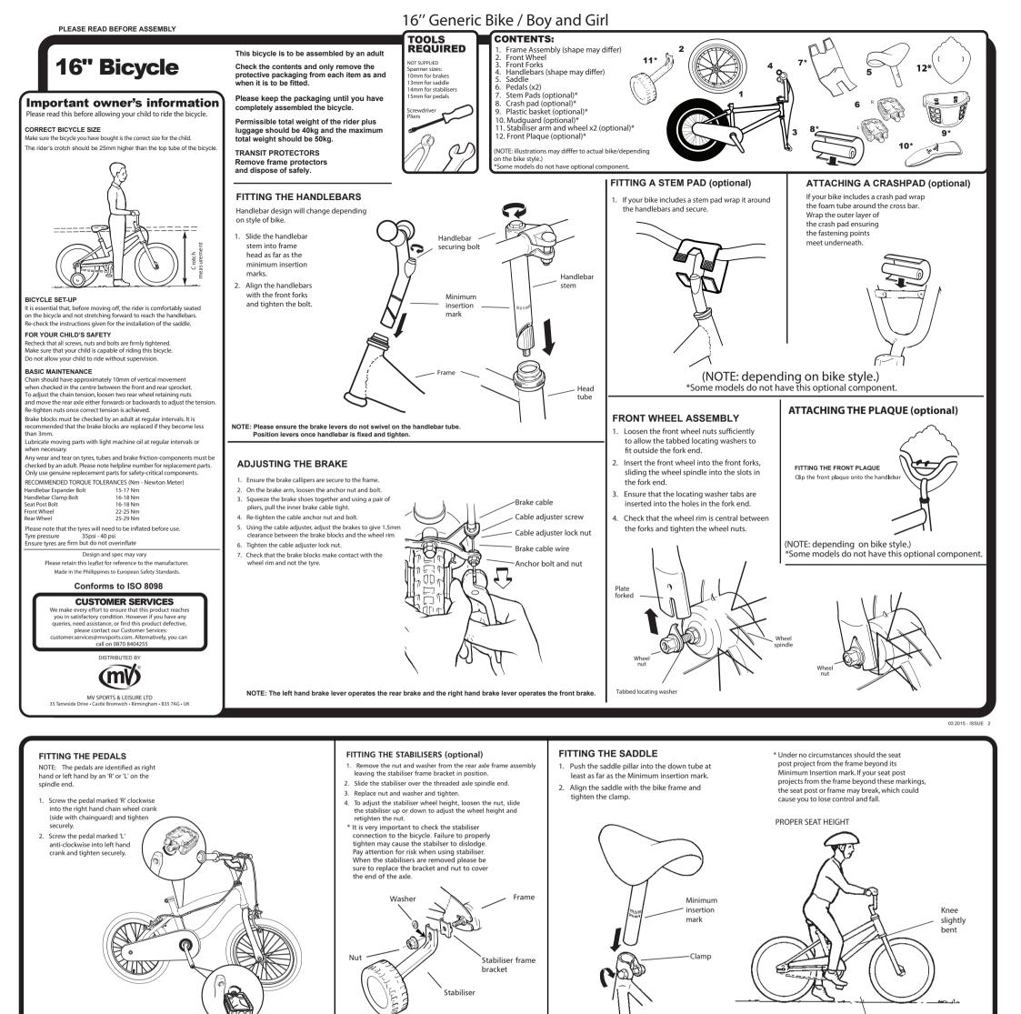
NOTE: Line up the pedal carefully with the hole in the wheel crank ensuring that it does not become cross threaded
