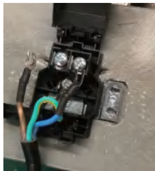
Fasten the wires beneath the screw heads
