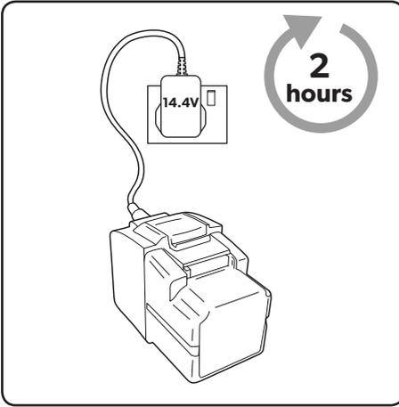
Plug the charger into the mains and connect it to the battery. Switch the power on at the mains.
