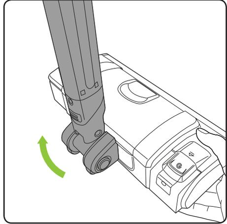
Lift the handle up to a 90° angle. The locking tabs on the steering module will slot in and you'll hear a 'click' when it's locked into place.
