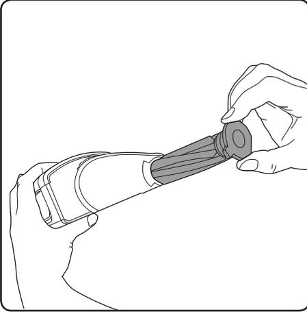
Pull the latch out to remove the brush-bar.
