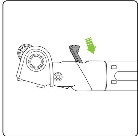
Make sure the handle is fully engaged with the steering module and push the locking clip into the handle. This will lock the handle into place.
