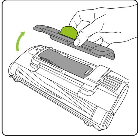
Lift and remove the bag-chamber lid.
