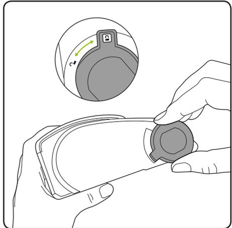
Remove the battery before maintaining any part of your HyLite. Rotate the latch from the 'locked' position to the 'unlocked' position.
