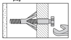
For use when fitting or supporting heavy loads such as shelving, wall cabinets and coat racks.
