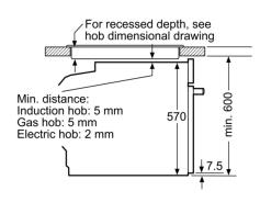
measurements in mm
