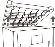
3. Remove the upper screws, then remove the upper hinge that hold the door in place. Lift the door and place it on a padded surface to prevent it from scratching.
