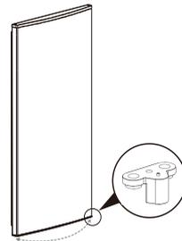
5. Remove the bottom screws, bottom hinge and levelling feet from the unit bottom.
