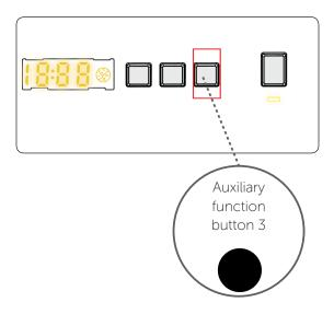
You can add an additional rinse operation to your laundry using this additional function. Your machine will carry out all rinsing steps with hot water. We recommend this setting for laundry worn on delicate skin, baby clothes and underwear.
