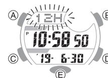
3. Press (D) to toggle the setting between [12H] (12-hour timekeeping) and [24H] (24-hour timekeeping).
