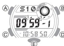
The watch beeps every second for the last five seconds of the current countdown, and starts the countdown of the next timer when the end is reached.
