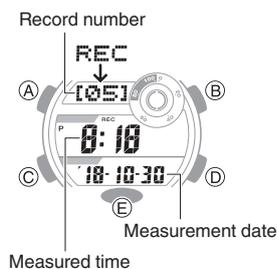
2. Press (A) to cycle through measurement numbers.
