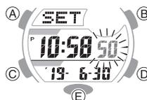
4. Hold down (E) for at least five seconds. Release the button when [RESET ALL] stops flashing.
