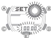
3. Press (C) eight times so [KEY↵] or [MUTE] is flashing on the display.
