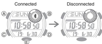
2. Hold down (D) for at least five seconds. Release the button when [FIND] starts to flash.
