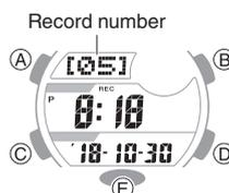
3. Hold down (D) and (E) at the same time for at least two seconds. Release the buttons when [CLR] stops flashing.
