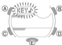
4. Press (D) to toggle the button operation tone between enabled and disabled.
