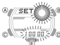
2. Keep pressing (C) until the setting you want to change is flashing.
