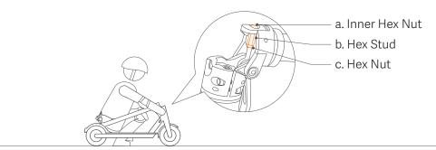
Long-term use of the scooter may result in loose screws, causing the handlebar stem to get unstable. If you notice the handlebar stem gets shaky when riding, follow the steps below.
