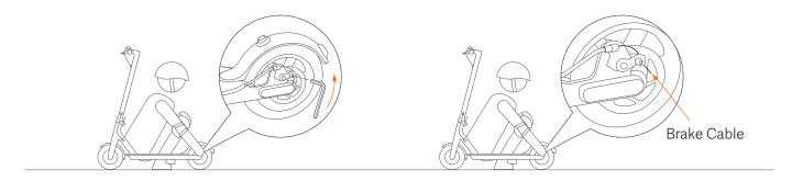
If the brake is too tight, use the 4 mm Allen key to loosen the screw on the caliper. Then slightly adjust the brake line (decrease the exposed length), and tighten the screw again.
