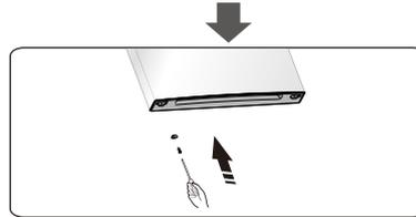
9. Change screw hole covers on middle cover plate from left to right (as shown in figure below).
