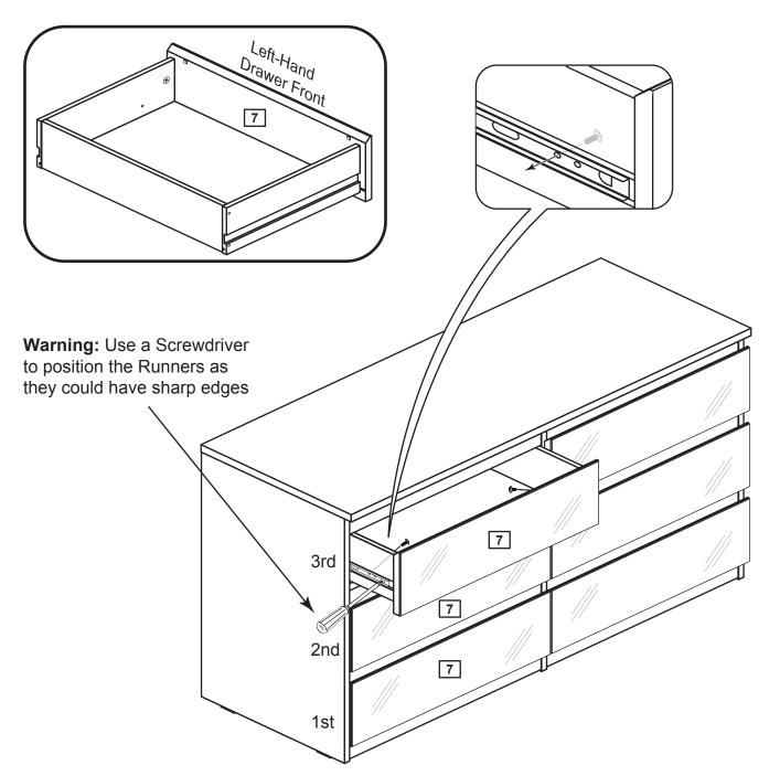
Starting with the bottom Left-Hand Drawer, slide both of the Runners forward and locate the Drawer Sides between them, lining up the holes in the Drawer Sides with the 2nd 'threaded' holes in the Runners.
