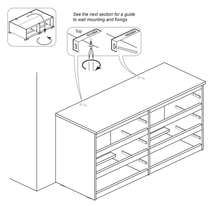
Slide the Brackets against the wall. Fit the 2nd screws supplied with the Brackets into the underside of the Top panel.
