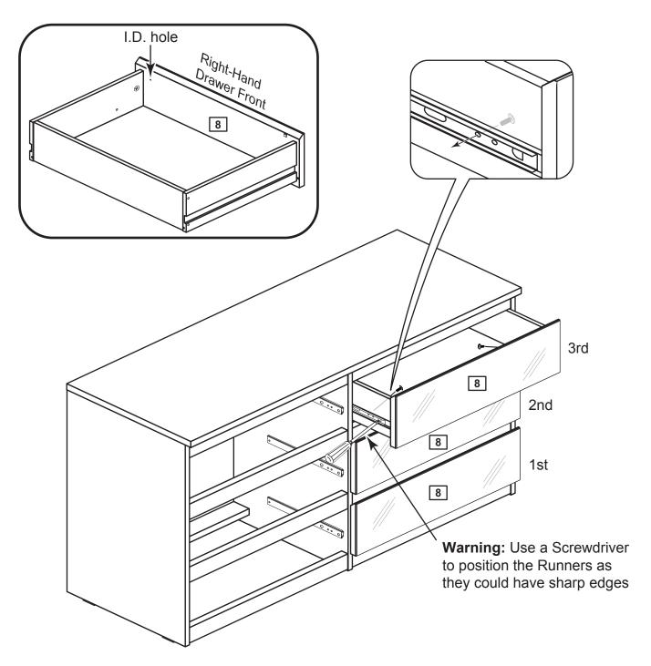
Starting with the bottom Right-Hand Drawer and working your way up, slide both of the Runners forward and locate the Drawer Sides between them, lining up the holes in the Drawer Sides with the 2nd 'threaded' holes in the Runners.
