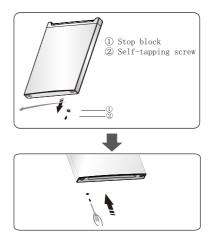
9. Change screw hole covers on middle cover plate from left to right (as shown in figure below).
