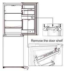
2. Use a putty knife or thin-blade screwdriver to prize the screw hole cover which is at the top left corner of the refrigerator, and the upper hinge cover which is at the top right corner of the refrigerator.
