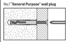
Generally aerated blocks should not be used to support heavy loads, use a specialist fitting in this case. For light loads, general purpose wall plugs can be used.
