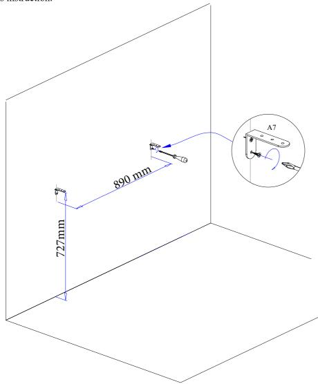
Attaching brackets to wall - please remember you must source and supply the fixings for attaching to your particular type of wall including the wall screws and wall plugs.
