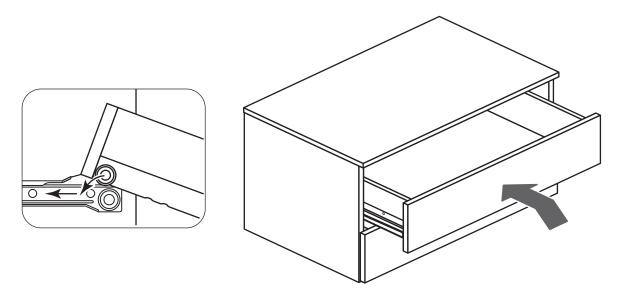
Insert the Drawers by sliding the wheels of the Runners fitted to the Drawers, over the wheels of the Runners fitted to the side panels and push the Drawers into position
