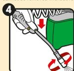
**SPRAY** - Adjust spray pattern by turning the nozzle. Aim 50 cm from target weed and press white trigger. Spray to lightly wet the leaves avoiding run off.
