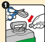
**CONNECT** - Cut the white tie to release the hose and wand. Connect the hose to the pack as shown. This is a quick couple system, so once in place it cannot be removed without force.
