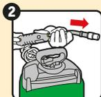
**EXTEND WAND** - Lift sprayer off the bottle, push the yellow button while pulling the lance into spray position.
