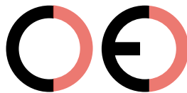
False CE Mark (too far)
