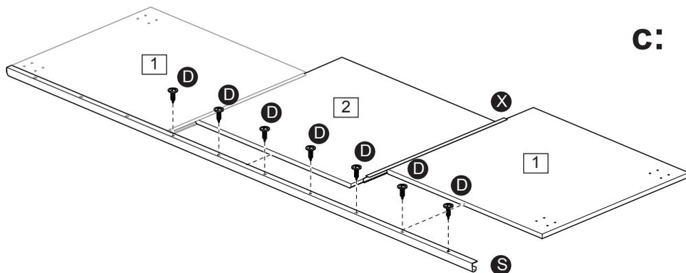
**d:** Mount door handle **S** on segment **1** with 4x screws **D** and on middle segment **2** with 3x screws **D**.
