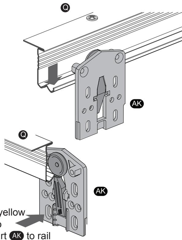
push the yellow lock pin to secure part **AK** to rail
