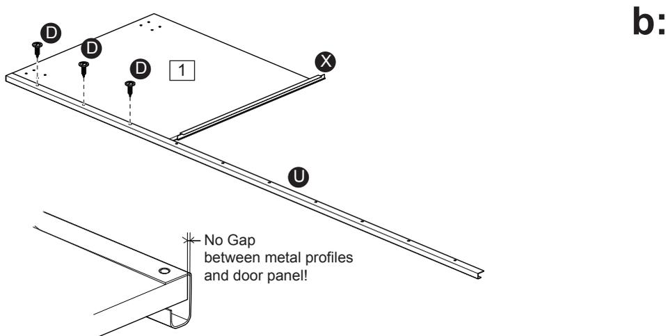
**c:** Mount segment middle **2** with 3x screws **D** on door trim **U**. Place 1x finishing profile **X** on segment **2**. Mount segment **1** with 4x screws **D** on door trim **U**.
