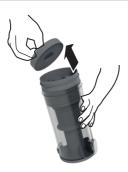
Remove the pre-motor filter from the bin (2).
