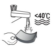
Wash the exhaust filter under warm water until the water runs clean (3).
