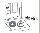
Remove excess water and leave to dry for 24hours (7). Only re-fit the filters when completely dry.
