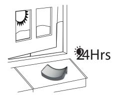
Remove excess water and leave to dry for 24hours (4). Only re-fit the filter when completely dry.
