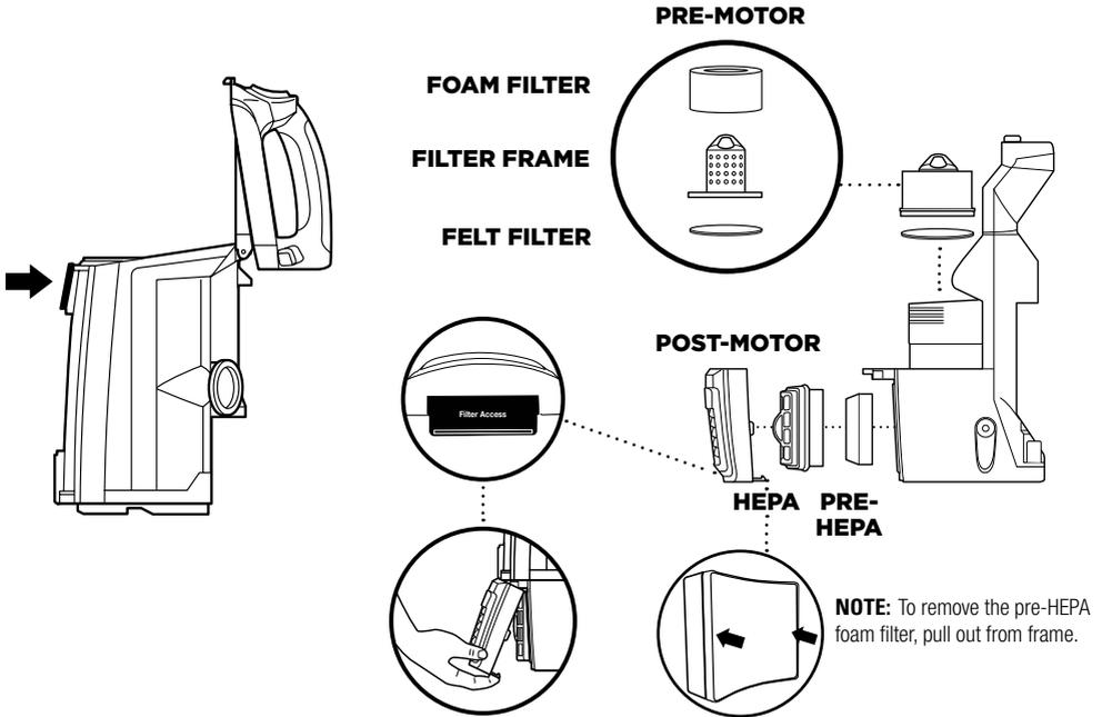
**3** Press top dust-cup empty latch to access dust screen and remove built-up debris as required.
