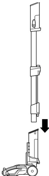
**1** Place motorised floor nozzle on floor and insert wand.
