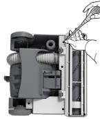
Remove the screws completely.
