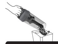
The dust container door will open and you can empty with no contact with dust.
