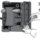
Refit sole plate opposite secure with screws.
