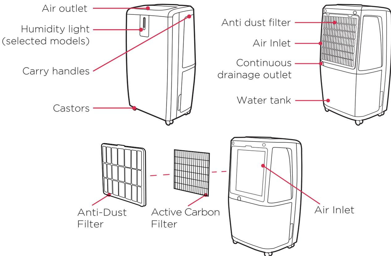
The Active Carbon Filter is used for capturing the smaller particles of dust suspended in the air and for tackling odours, absorbing formaldehyde, benzene and other noxious gases.
