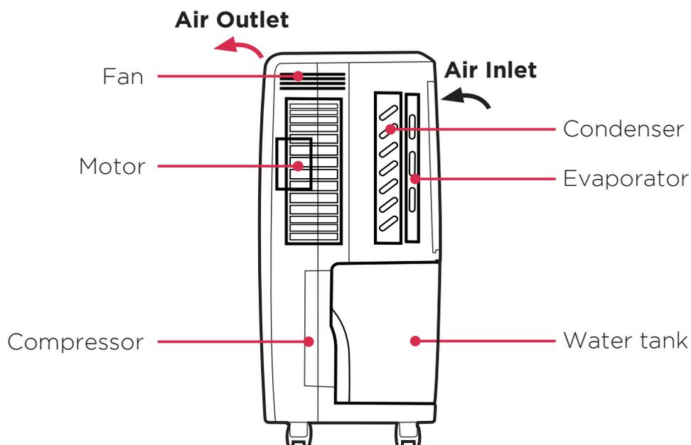
This product is a dehumidifier. It controls relative humidity by passing the air through the unit, forcing the excess moisture to condensate over the cooling elements.
