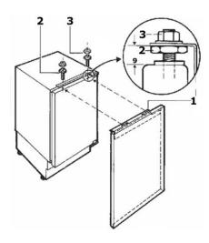
3. Hang the furniture door onto the appliance door, making sure that the brackets on the mounting bracket locate over the adjusting bolts.
