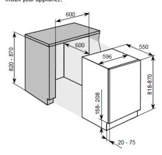
o The appliance must be stood on a level floor. You can use the levelling feet to take into account any minor unevenness in the floor.
