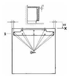
Measure the width of the furniture door, at the halfway point mark a line vertically down the inner surface of the furniture door. You should draw the line from the top of the furniture door to approximately halfway down.
