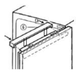
Insert the cover plate to the top of the appliance, this will just clip into place.
