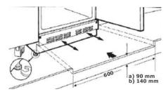
o Use a spanner to adjust the height of the adjustable feet.
