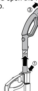
5 Connect the hose to the handle tube. Connect the accessory to the handle tube.
