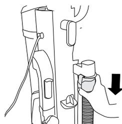
3 Plug the lower hose end in the hose socket.
