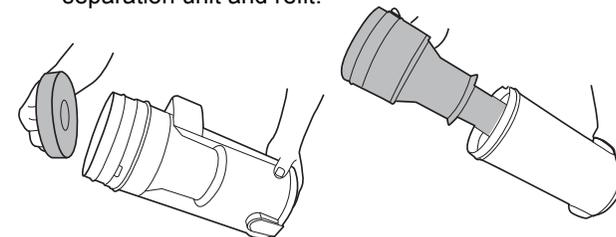
**4** Wash both filter and sponge under warm water until the water runs clean. Remove excess water by shaking and leave to dry for 24 hours. Reassemble and refit filters to cleaner, only when they are completely dry.
