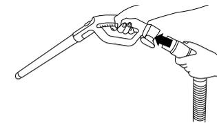
The hose can be removed at both ends.
