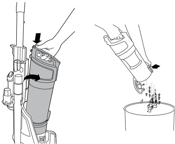
**1** To remove the bin from the cleaner press the bin release button.
