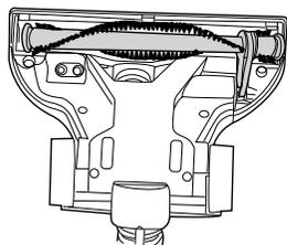
**NOTE:** When the brush bar is blocked, the nozzle will stop rotating and nozzle LED will be flashing. Switch off and remove the plug from the electricity supply, then use a pair of scissors to cut through any threads or hairs embedded around the brush bar. Reassemble the brush bar and the brush guard.
