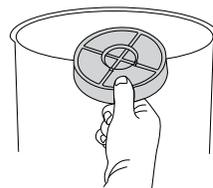
**2** Take out the pre motor filter and the separation unit from the dust bin. Clean excess debris from the separation unit and refit.
