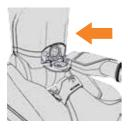
Push hose end and hose solution connector into connection port until it clicks into place.
