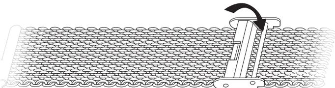
3. Close metal plate, locking the pin-bar half of the clasp in new position on the bracelet.
