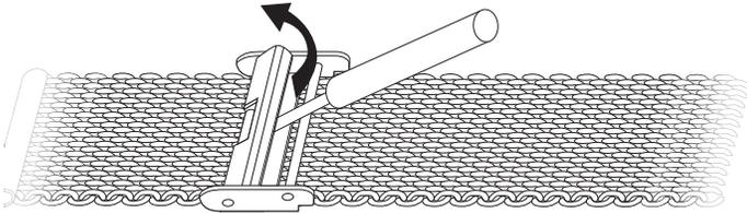
1. Use tool such as a small flat-head screwdriver to pop open metal plate on pin-bar half of clasp, releasing the clasp position locking mechanism.
