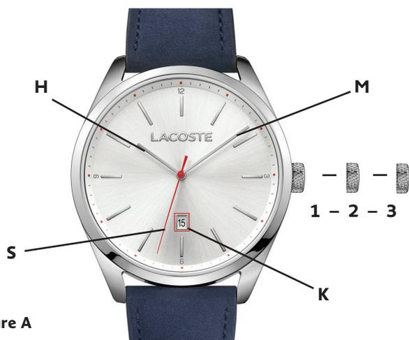
**Power depletion warning function:** When the battery nears its end, the second hand moves at two-second intervals instead of the normal one-second intervals. In that case, have the battery replaced with a new one as soon as possible. The watch remains accurate while the second hand is moving at two-second intervals.
