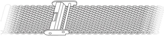
Above: Open mesh bracelet side with pin-bar half of sliding clasp locked in position.
