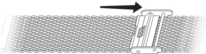
2. Slide pin-bar half of clasp along the mesh bracelet in either direction to desired position.
