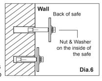
Please note that the wall bolts are only to be used in brick & cement structures.
