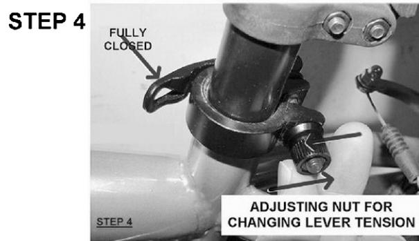
**IF THE SEATPOST / SADDLE IS NOT SECURE ENOUGH, FLIP LEVER TO OPEN POSITION AND SLIGHTLY TIGHTEN ADJUSTING NUT AND FLIP LEVER TO CLOSE POSITION AND CHECK. REPEAT UNTIL SEATPOST IS VERY SECURE. AS A GUIDE THERE SHOULD BE ENOUGH TENSION TO MAKE LEVER HARD TO FLIP CLOSED**
