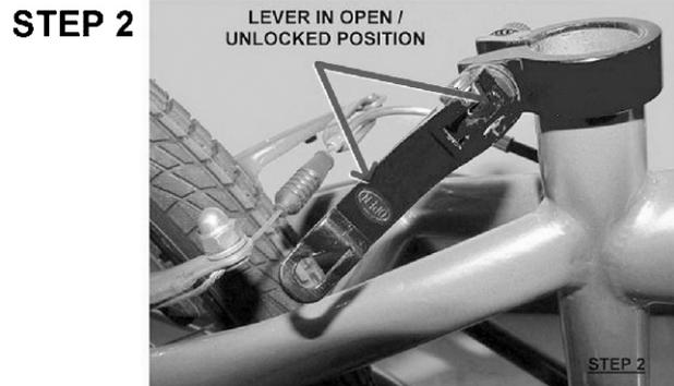
**THE QUICK RELEASE CLAMP IS MARKED OPEN & CLOSED. WHEN IN OPEN POSITION, SEAT POST CAN BE INSERTED INTO THE FRAME TO THE DESIRED HEIGHT POSITION**
