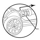
Ensure the 'handlebar lock' springs back to lock in position.
