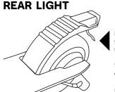
Remove the thin plastic strip from under the light unit, to activate the battery.
