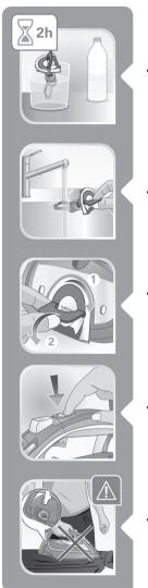
• To descale the Micro Calc filter thoroughly rinse it in diluted citric acid for 2 hours.
