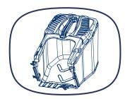
ii. Lift up the rear flap before assembling the grass bag. Hang the collection bag on the mower.
