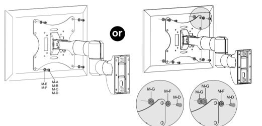
The spacers illustrated above are optional and should be used if the back of your TV is not flat to compensate and provide a solid mounting surface.
