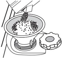
1. Remove the lower rack and unscrew the reservoir cap (an anticlockwise).
