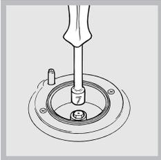
Replacing the nozzles for the hob burners:
