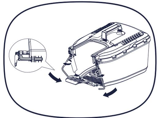
iii. To remove the mulching plug, grip the post and squeeze the lever, push down (1) to release the catch (2). Once the catch is released the mulching plug can be lifted out of the mower (3).
