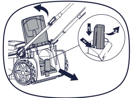
iv. Ensure the mulching plug is removed from the lawnmower before fitting the grass collection bag. Lift up the deflector guard all the way up with one hand and attach the grass collection bag onto the mounting brackets provided at the rear of the mower. Align the bottom of the grass collection bag first ensuring the collection tongue is located fully within the discharge chute of the lawnmower. Lower the deflector guard.
