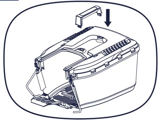
ii. Secure the metal support rods into the fixing position on either side of the grass collection base. Ensure the side clamping sleeves are properly fixed onto the metal support frame.
