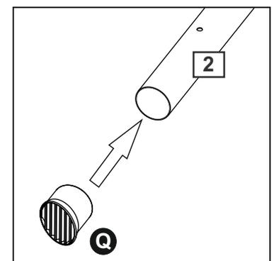
b: Insert the plastic foot **Q** onto the other end of the front legs **2**
