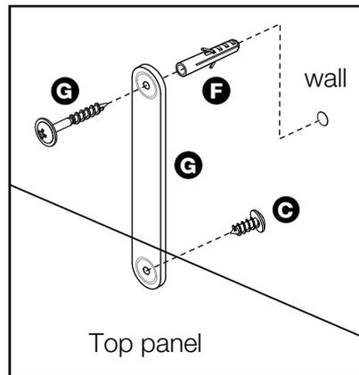
**Note:** Wall plugs supplied are for solid wall only. The correct type of fixing must be used for your wall, seek professional advice if in doubt
